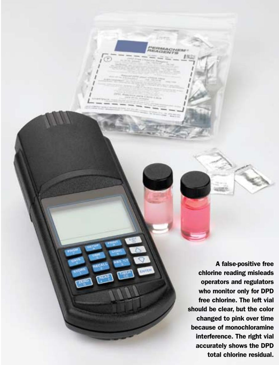
**A false-positive free chlorine reading misleads operators and regulators who monitor only for DPD free chlorine. The left vial should be clear, but the color changed to pink over time because of monochloramine interference. The right vial accurately shows the DPD total chlorine residual.**
